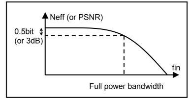
sample and hold, dc input may show full 8-bit performance even at the maximum sample rate of 200M sample/s. However, a high-frequency sinusoidal input at, say, 40MHz, will require the input stage to track a rapidly varying signal and may result in only 6-bit performance.
