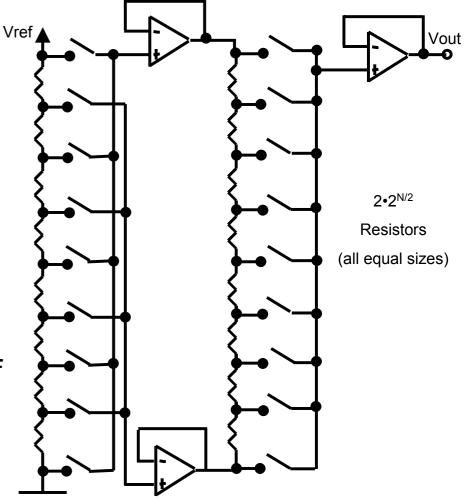
The second resistor string is used to decode only lower-order bits
